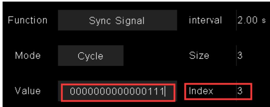
In cycle mode, signals will output in turn.
