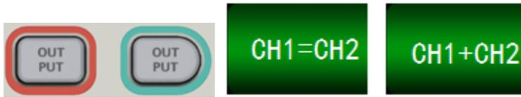
CH1=CH2: The output signal of CH1 is the same as the output signal of CH2.
