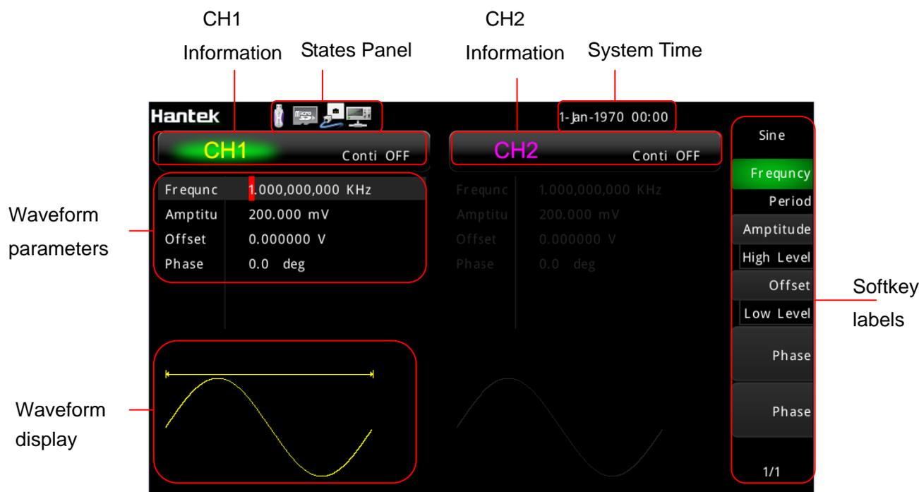
Status panel indicates whether external usb device is connected with this device, whether usb device in the rear panel is connected with PC, whether the Internet is connected and the current time.
